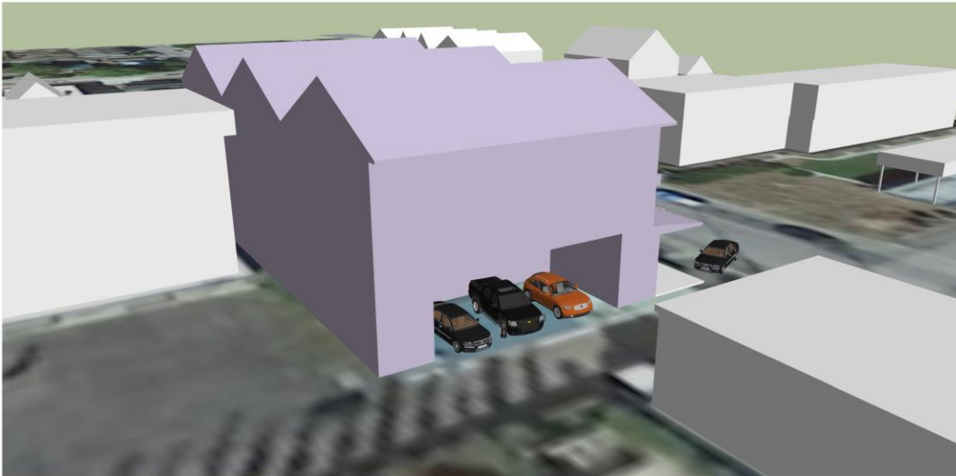
Covered parking for loading and unloading is easily accessed from the alley and is recessed into the building.
